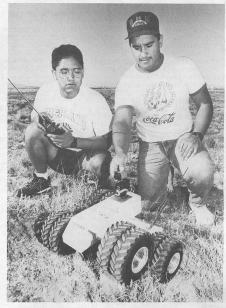
THIS RATLER DOESN'T BITE - Students Leon Martine (left) and Adan Delgado (both 9616) prepare to put a model of Sandia's Robotic All-Terrain Lunar Exploration Rover (RATLER) through its paces traversing rugged rocks and hills around Sandia's Robotic Vehicle Range. RATLER is Sandia's first of a new breed of space robots known as micro-rovers designed to have a small launch mass and yet large payload capacity. (Photo by Randy Montoya)
